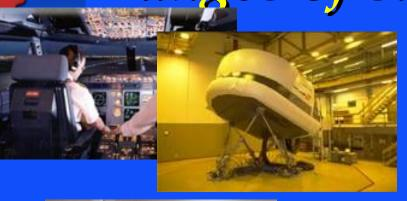
These \$10MM flight simulators are used to train airline pilots from around the world and they exactly replicate the flight deck of the real aircraft, with sophisticated views of the outside world.
