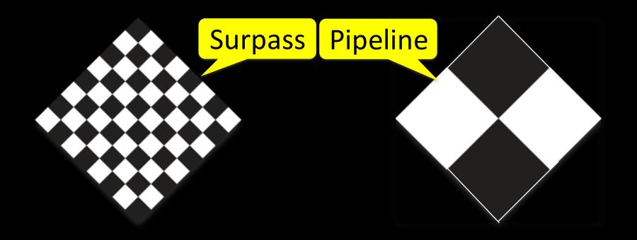
Schematic showing equal porosity (50%) but different mesh densities
