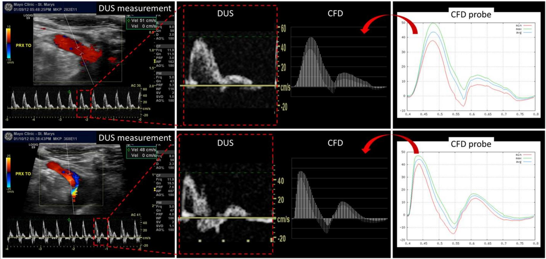
→ Consistent flow waveforms and peak velocities
