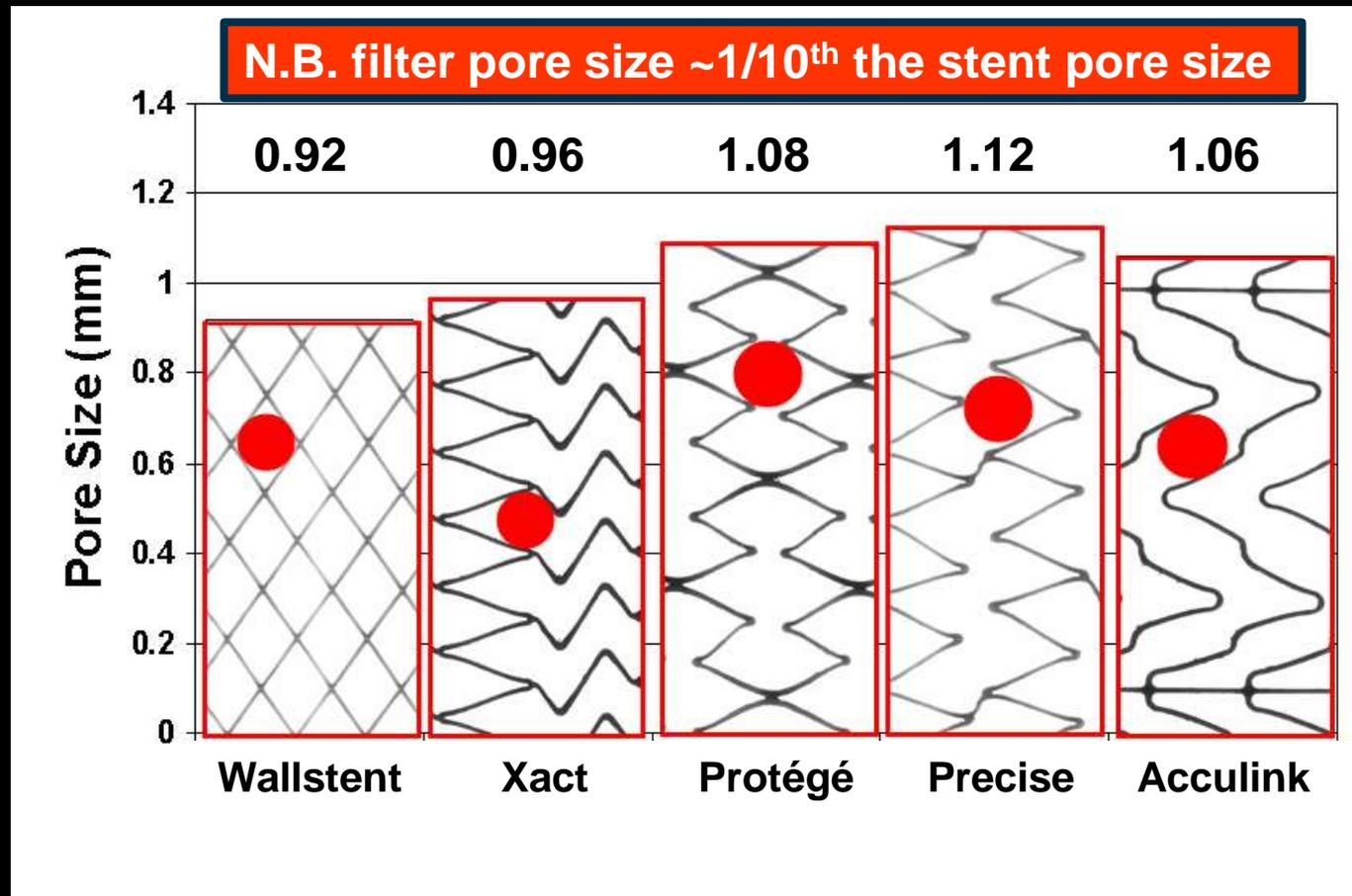
Xact, PROTÉGÉ RX and Acculink = 8-6mm tapered stents (distal portion)
